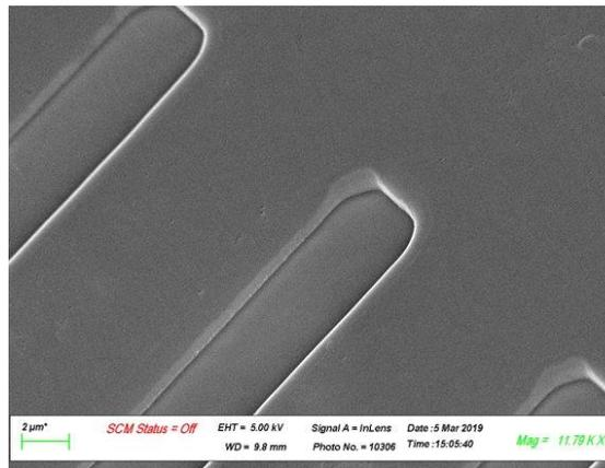
“ADAMA innovations IIL structured grating, replicated by PROMOLDING with their injection moulding machines”.
